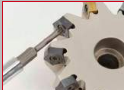
Long bit for traditional mounted inserts.
