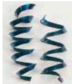
Too long: May clog drill flutes. Reduce speed or increase feed within recommended limits.
