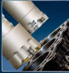
Machining of cylinder crank cases
